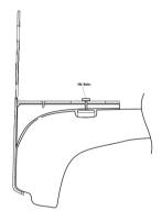
13. Fit awning to awning mount using the bolts provided with awning and tighten to specs within awning instructions.
