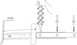
10. Measure and cut the rubber roof trim with tin snips and put back in the vehicle roof channel at the front, middle and rear of the tracks, the front piece needs to be measured so the end of the trim sits under the windscreen rubber.
