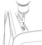
NOTE: USE CARE WHEN BREAKING THROUGH. A DRILL STOP IS RECOMMENDED Use a vacuum to remove swarf from the roof channel.
