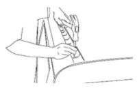
Marked out holes can now be drilled using a 5mm drill bit with a drill stop. Set up the drill stop ensuring you don't drill through the roof lining.
