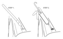
8. Accurately place the mount over the drilled holes in the roof channel using the rivets to position.
