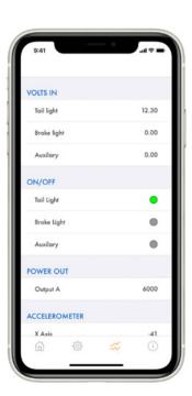
When brake pedal pressed the voltage indicator responds with voltage value.
