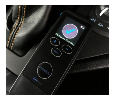
4. When braking in the vehicle the remote will indicate red that the trailer is performing a brake response.
