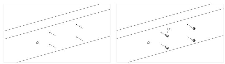
1. Pre-drill holes using 2-3 mm drill.
