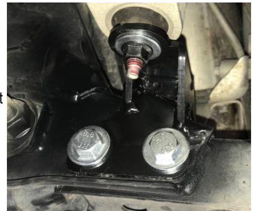
FIG 4&5. Fit bracket as shown in images using the 2 x M10x1.50P x 110mm long bolts with M10 Flange nuts and washers supplied. Reinstall factory bolt through diff mount into new bracket, fit supplied washer and flange nut, leave loose until the end of installation procedure.
